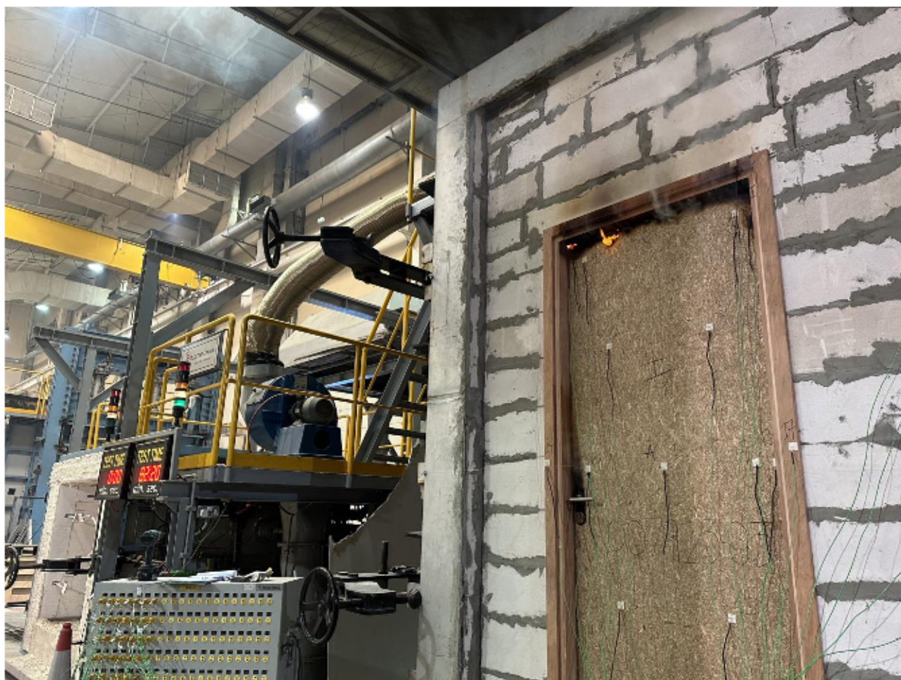
Photo 2. At 82:20 minutes after Door #1 has failed due to sustained flaming.
